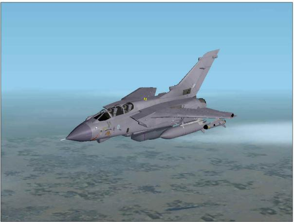
When the wings are swept back, the Tornado GR4 increases its high-speed low-level capability by reducing drag. When sweeping, the wings partially slide into the fuselage, reducing the exposed wing area. This gives the aircraft a low gust response in turbulent low-level winds. This not only makes flight much more comfortable for the aircraft a more stable platform from which to aim and deliver unguided weapons at low level.
