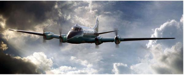
they basically enlarged the Dove; lengthened the fuselage in order to provide room for more passengers or freight, and increased the wingspan to make room for two additional engines. The resulting aircraft was supposed to be able to use many of the parts originally designed for the Dove, thus simplifying logistics for airlines employing both types.
