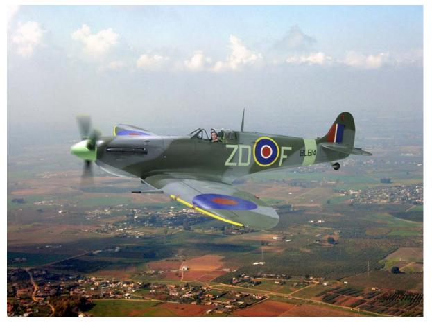
The elliptical wing was chosen for superior aerodynamic attributes but it was a complex wing to construct and the Messerschmitt Bf 109's angular and easy-toconstruct wing offered similar performance (model per model) to the Spitfire. It has been reported that the Bf 109 took one-third the man hours to construct compared to the Spitfire.
