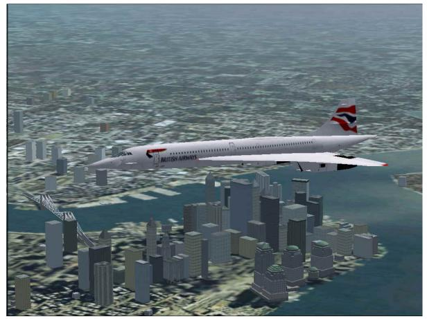
cruise speed of Mach 2.02 (about 2,140 km/h or 1,330 mph) with a maximum cruise altitude of 60,000 feet (18,300 metres), rather more than twice the speed of conventional aircraft. The average landing speed was a relatively high 185 mph (160 knots).
